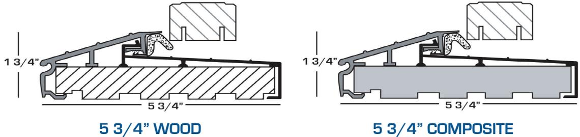
PVC internal crown accepts standard 1 1/2", 2", 2 3/4" and 4" aluminum sill extension.
